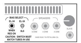
**NOTE:** It is extremely important that the **BIAS SWITCH** setting match the type of tubes in use. Failure to comply will result in damage to your amplifier. Always check the **BIAS SWITCH** whenever swapping tubes!
